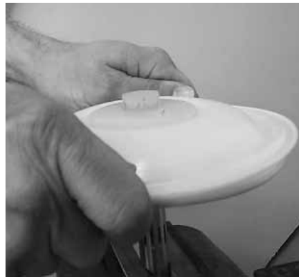
Step 13. Figure 13 To remove the remaining diaphragm assembly from the shaft, secure shaft with soft jaws (a vise fitted with plywood or other suitable material) to ensure shaft is not nicked, scratched, or gouged. Using hands or an adjustable wrench, remove diaphragm assembly from shaft. Inspect all parts for wear and replace with genuine Wilden parts if necessary.
